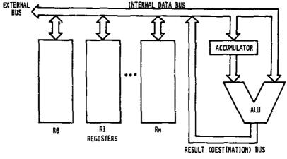
Fig. 2.8: Single-Bus Architecture
