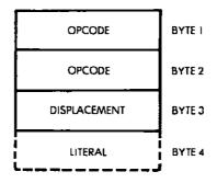
Fig. 5.5: Indexed Addressing Has 2-byte Opcode
