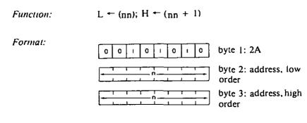
Description: The contents of the memory location addressed by the memory locations immediately after the opcode are loaded into the L register. The contents of the memory location after the one loaded into the L register are loaded into the H register. The low byte of the nn address occurs immediately after the opcode.
