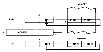
Fig. 4.13: Digit Rotate Instructions (Rotate Decimal)
