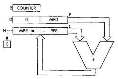
Fig. 3.25: Registers for Improved Multiply
