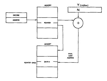
Fig. 5.3: Indirect Indexed Addressing (Post-Indexing)
