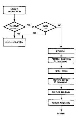
Fig. 6.34: Interrupt Logic
