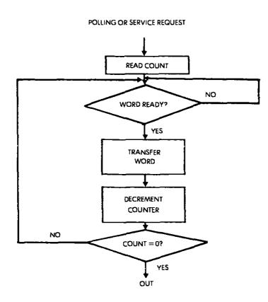
Fig. 6.5: Parallel Word Transfer: Flowchart
