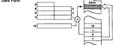
Timing: 5 M cycles; 19 T states; 9.5 usec @ 2 MHz
