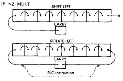
Fig. 3.17: Shift and Rotate
