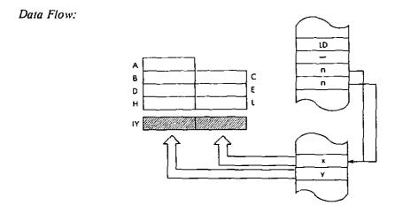
Timing: 6 M cycles; 20 T states; 10 usec @ 2 MHz
