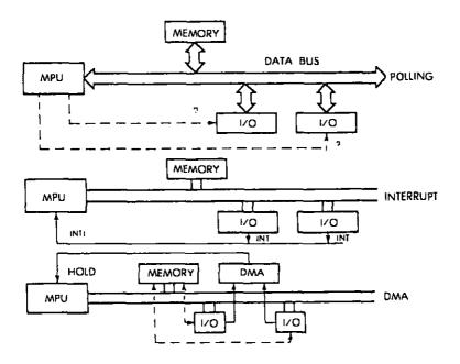
Fig. 6.18: Three Methods of I/O Control
