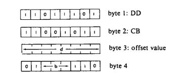
Description: The specified bit of the memory location addressed by the contents of the IX register plus the given offset value is tested and the Z flag is set according to the result. b may be any one of:
