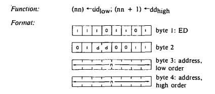
The contents of the low order of the specified Descriptions: register pair are loaded into the memory location addressed by the memory locations immediately following the opcode. The contents of the high order of the register pair are loaded into the memory location immediately following the one loaded from the low order. The low order of the nn address occurs immediately after the opcode.dd may be anyone of:
