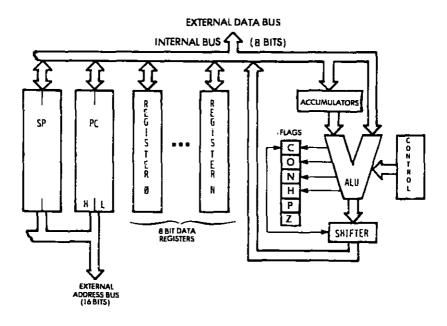
Fig. 2.2: "Standard" Microprocessor Architecture
