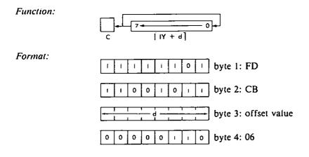
Description: The contents of the memory location addressed by the contents of the 1Y register plus the given offset value are rotated left and the result is stored back at the location. The contents of bit 7 are moved to the carry flag as well as bit 0.
