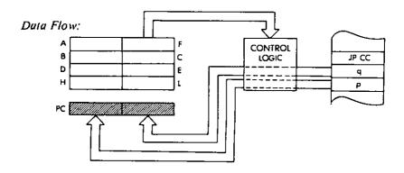
Timing: 3 M cycles; 10 T states; 5 usec @ 2 MHz
