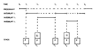
Fig. 6.33: Stack Contents During Multiple Interrupts
