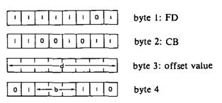
Description: The specified bit of the memory location addressed by the contents of the IY register plus the given offset value is tested and the Z flag is set according to the result. b may be any one of:
