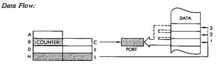
Timing: B = 0: 4 M cycles; 16 T states; 8 usec @ 2 MHz. $B \neq 0: 5 \text{ M cycles}; 21 \text{ T states}; 10.5 \text{ usec } @ 2 \text{ MHz}$
