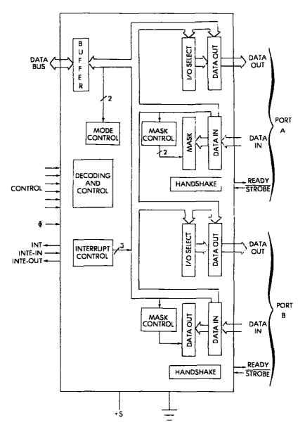
Fig. 7.7: Z80 PIO Block Diagram
