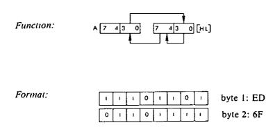
Description: The 4 low order bits of the memory location addressed by the contents of HL are moved to the high order bit positions of that same location. The 4 high order bits are moved to the 4 low order bits of the accumulator. The low order of the accumulator is moved to the 4 low order bits of the memory location originally specified. All of these operations occur simultaneously.
