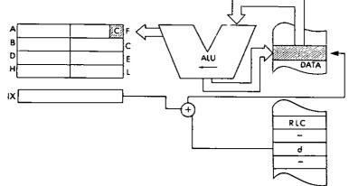
Timing: 6 M cycles; 23 T states; 11.5 usec @ 2 MHz
