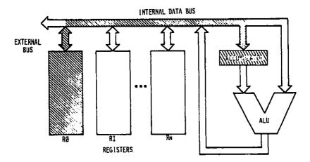
Fig. 2.9: Execution of an Addition-R0 into ACC
