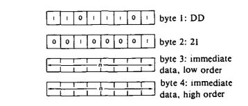
Description: The contents of the memory locations immediately following the opcode are loaded into the IX register. The low order byte occurs immediately after the opcode.
