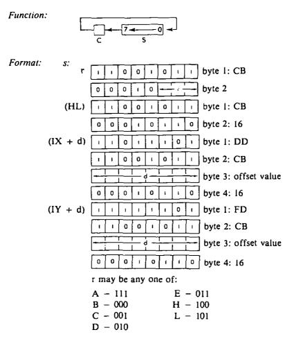
Description: The contents of the location of the specific operand are shifted left one bit place. The contents of the carry flag are moved to bit 0 and the contents of bit 7 are moved to the carry flag. The final result is stored back in the original location. s is defined in the description of the similar RLC instructions,
