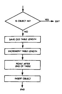
Fig. 9.13: Table Insertion Flowchart
