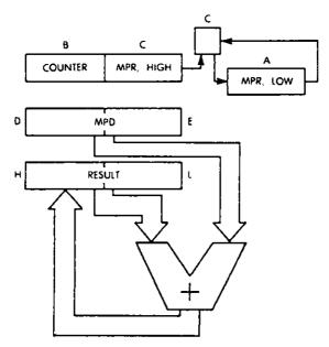
Fig. 3.27: 16 × 16 Multiply—The Registers
