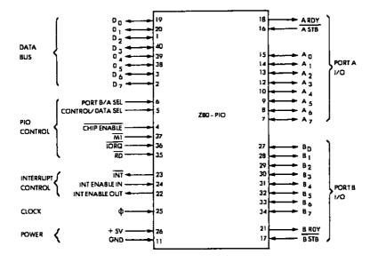
Fig. 7.6: Z80 PIO pinout
