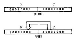
Fig. 2.20: Transferring C into D
