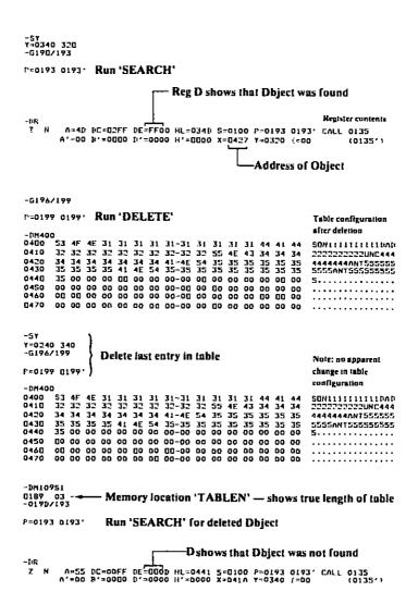
Fig. 9.17: Simple List- A Sample Run (cont.)
