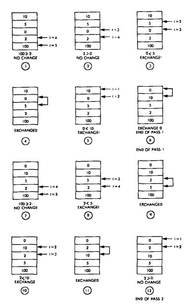
Fig. 8.5: Bubble-Sort Example: Phases 1 to 12
