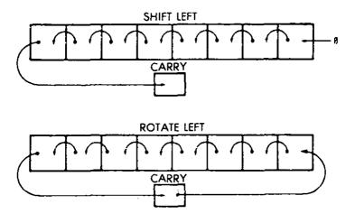
Fig. 4.1: Shift and Rotate
