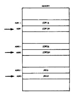
Fig. 3.7: Pointing to the High Byte
