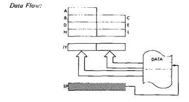
Timing: 4 M cycles; 14 T states; 2 usec @ 2 MHz
