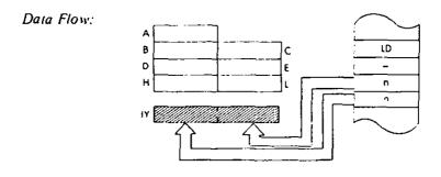
Timing: 4 M cycles; 14 T states; 7 usec @ 2 MHz
