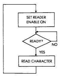
Fig. 6.20: Reading from a Paper-Tape Reader
