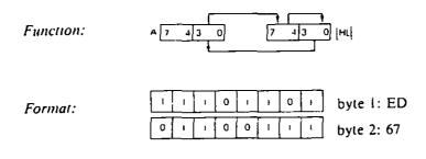
Description: The 4 high order bits of the memory location addressed by the contents of the HL register pair are moved to the low order 4 bits of that location. The 4 low order bits are moved to the 4 low order bits of the accumulator. The low order bits of the accumulator are moved to the 4 high order bit positions of the memory location originally specified. All of the above operations occur simultaneously.
