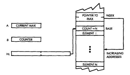
Fig. 8.1: Largest Element in a Table
