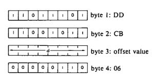
Description: The contents of the memory location addressed by the contents of the IX register plus the given offset value are rotated left and the result is stored back at that location. The contents of bit 7 are moved to the carry flag as well as to bit 0.
