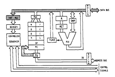
Fig 2.18: PC Is Incremented
