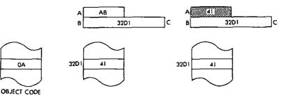
LD A, (DE) Load the accumulator from the memory location indirectly addressed by the DE register pair.
