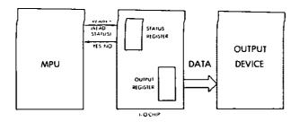
Fig. 6.8: Handshaking (Output)
