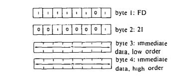
Description: The contents of the memory locations immediately following the opcode are loaded into the IY register. The low order byte occurs immediately after the opcode.
