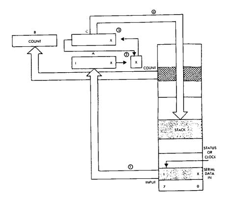
Fig. 6.7: Serial-to-Parallel: The Registers
