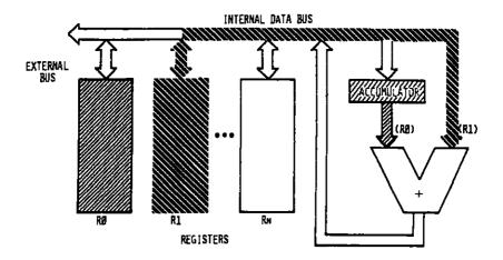
Fig. 2.10: Addition-Second Register R1 into ALU
