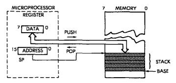
Fig. 2.5: The Two-Stack Manipulation Instructions
