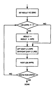
Fig. 3.12: The Basic Multiplication Algorithm-Flowchart
