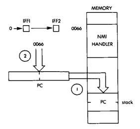
Fig. 6.25: NMI Forces Automatic Vectoring
