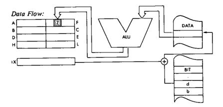
Timing: 5 M cycles; 20 T states: 10 usec @ 2 MHz
