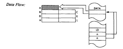
Timing: 4 M cycles; 13 T states; 6.5 usec @ 2 MHz
