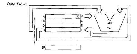
Timing: 4 M cycles; 15 T states; 7.5 usec @ 2 MHz
