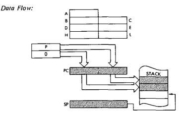
Timing: 3 M cycles; 11 T states; 5.5 usec @ 2 MHz
