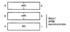
Fig. 3.29: 16  $\times$  16 Multiply with 32-Bit Result
