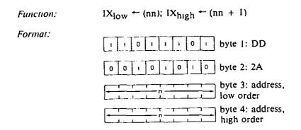
Descriptions: The contents of the memory location addressed by the memory locations immediately following the opcode are loaded into the low order of the IX register. The contents of the memory location immediately following the one loaded into the low order are loaded into the high order of the IX register. The low order of the nn address immediately follows the opcode.
