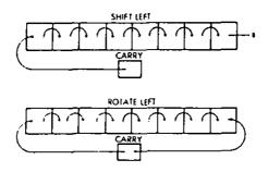
Fig. 4.9: Shift and Rotate
