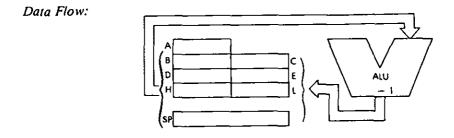
1 M cycle; 6 T states; 3 usec @ 2 MHz Timing:
