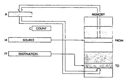
Fig. 5.7: Block Transfer: Initializing the Register
