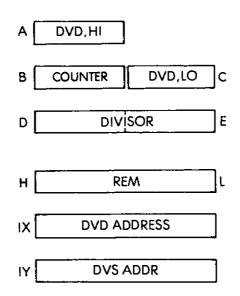
Fig. 3.34: Non-Restoring Division—The Registers
