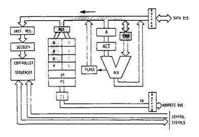
Fig. 2.22: The Contents of TMP are Deposited into D
