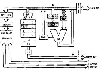
Fig. 2.23: Two Transfers Occur Simultaneously
