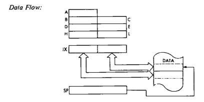
Timing: 6 M cycles; 23 T states; 11.5 usec @ 2 MHz
