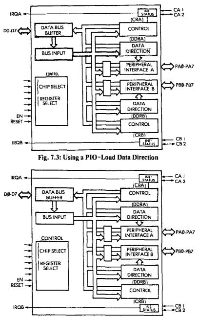
Fig. 7.4: Using a PIO-Read Status
