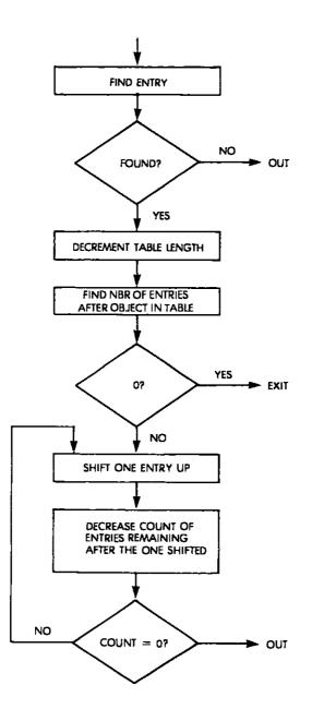
Fig. 9.15: Table Deletion Flowchart
