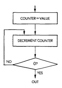
Fig. 6.3: Basic Delay Flowchart
