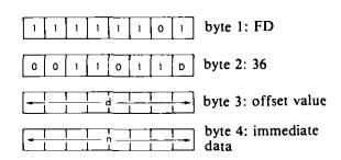
Description: The contents of the memory location immediately following the offset are transferred into the memory location addressed by the contents of the index register plus the given offset value.
